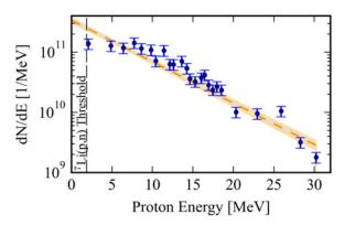
FIGURE 3. Measured proton energy spectrum. The circles show the proton spectrum inferred using RCF and the dashed line is a decaying exponential, with parameters  $N_0 = 2.14 \times 10^{12}$ , T = 6.3 MeV and  $E_{\text{max}} = 30.5$  MeV. The solid background shows the region of calculated uncertainty within one standard deviation of  $1.3 \times 10^{11}$  for  $N_0$  and 0.2 MeV for T.
