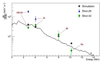
FIGURE 14. Neutron energy spectrum at  $0^{\circ}$ . The dark line shows the spectrum determined from the Geant4 simulations which has been normalized by the number of neutrons observed from the <sup>7</sup>Be residual (i.e. 2 times). The different markers represent the average energies and neutron fluences for individual samples as described in the text.
