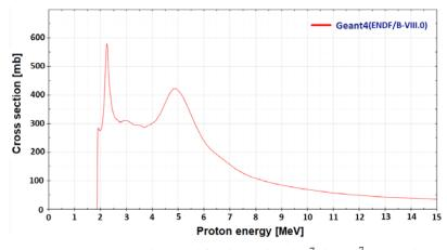
FIGURE 4. Cross-section used for simulating the  $^{7}$ Li(p,n) $^{7}$ Be reaction.
