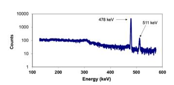
FIGURE 7. Activation spectra of the LiF using the onsite high-purity Ge. The 478 and 511 keV lines are from the <sup>7</sup>Be decay and electron–positron annihilation, respectively.
