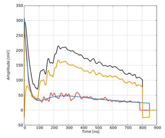
FIGURE 11. Background subtraction procedure in the experiment for Detector 10, with a 30 cm thick front Pb shielding: (black) nToF for the detector in the shot of interest after the  $\gamma$ -peak time alignment; (red) background distribution from a shot with the LiF secondary target removed; (blue) fit of the background distribution; (yellow) background-subtracted nToF distribution for the detector.
