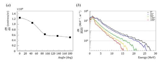
FIGURE 6. The neutron yields (*a*) and neutron spectra (*b*) at different angles as found from Geant4 simulations.
