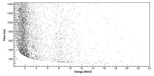
FIGURE 10. Relationship between the simulated time-of-flight distribution and the initial energy of the neutrons, for Detector 10, with a 30 cm thick front Pb shielding.
