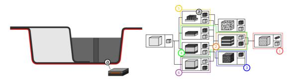
1 Layer manufacturing 2 Prepreg pressing 3 Foam core manufacturing 4 Bonding of shells and foam 6 Coating by injection moulding 5 Injection moulding of ribbing
