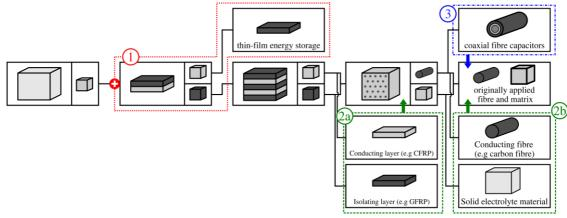
Figure 3. Example of a multi-level structure at the example of a integration of a structural battery into FRP on different level applied to the example of Adam et al. (2018)
