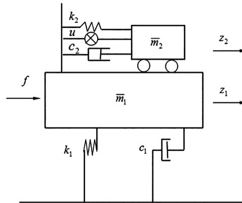
FIGURE 1. An offshore platform with an AMD mechanism [2].
