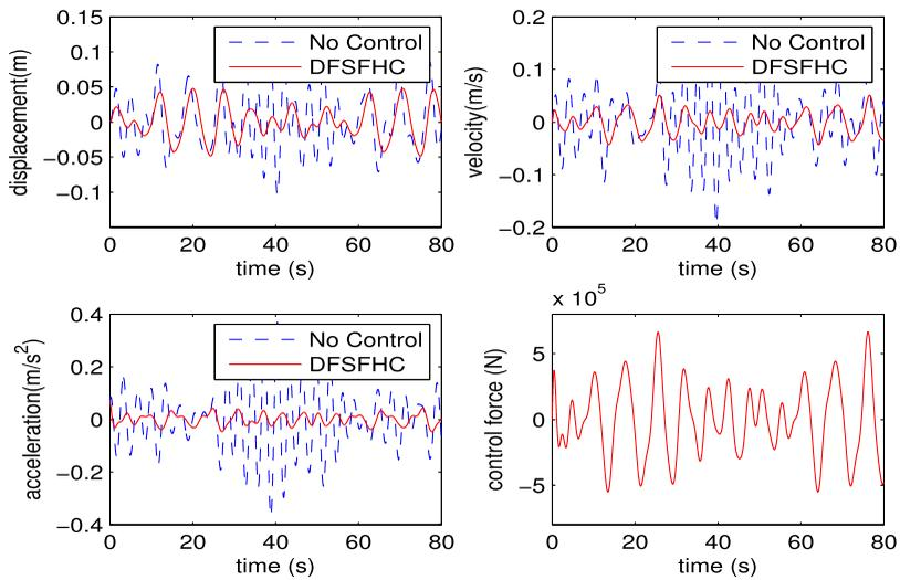
FIGURE 2. Responses of offshore platform and control force. (Colour available online).
