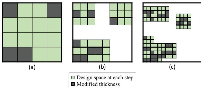
**Figure 2.** The stepwise design space discretisation for topometry optimisation, (a) discretised design space at step 1, (b) discretised design space at step 2, (c) discretised design space at step 3
