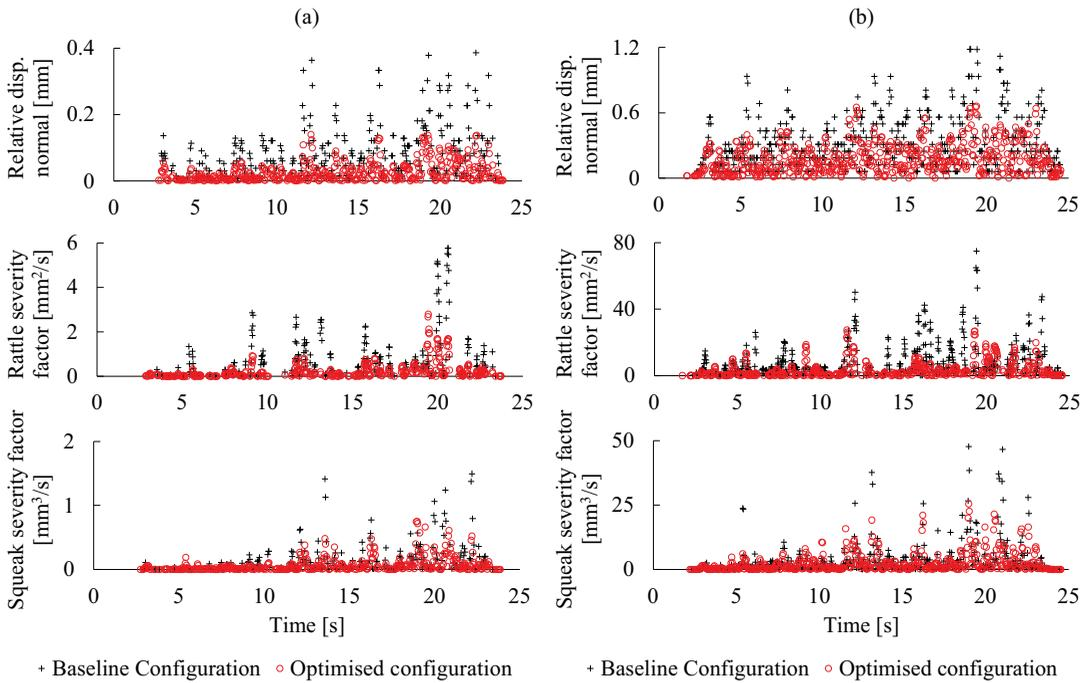
**Figure 11.** Relative displacement and squeak and rattle severity factors for the baseline and optimised designs excited by Pave disturbance at the (a) top-left measure point and (b) bottom-right measure point of the inner door panel.
