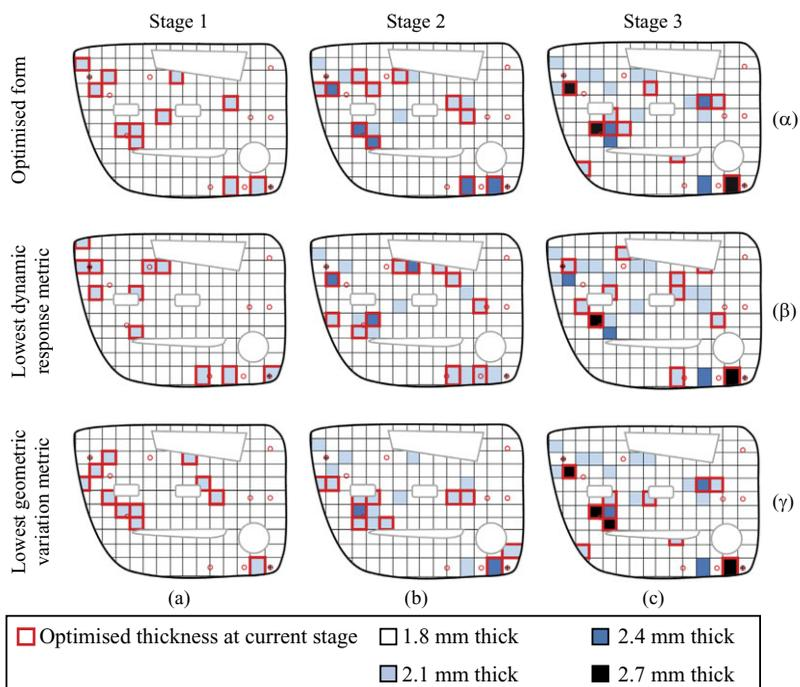
**Figure 10.** The schematic thickness variation for (a–c) the results at different optimisation stages, ( $\alpha$ ) the selected designs at each stage as the optimised design and ( $\beta$ – $\gamma$ ) in selected designs from the Pareto front in Figure 9.
