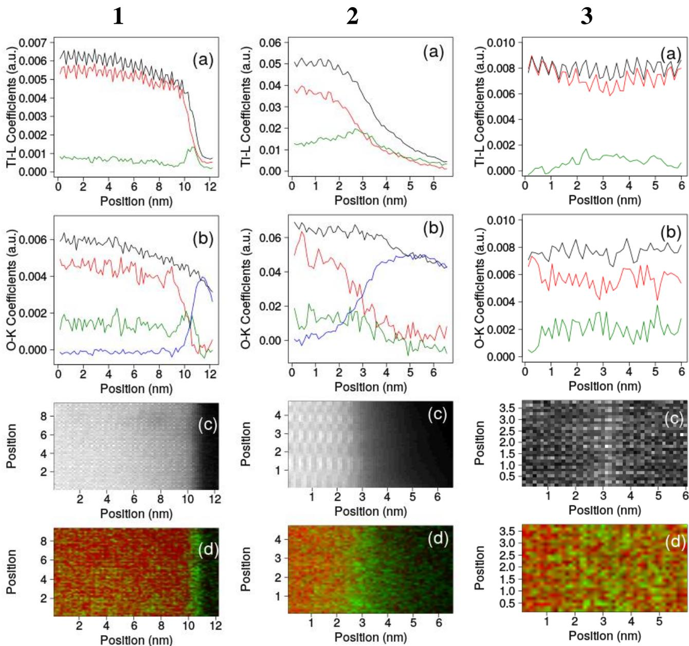
**Figure 1.**  $\gamma$ -Al<sub>2</sub>O<sub>3</sub>/SrTiO<sub>3</sub> sample grown by ALD at 345 °C with 2DEG density of  $6 \times 10^{13}$  cm<sup>-2</sup> at room temperature. (a) Fitting coefficients from Ti-L edge. (b) Fitting coefficients from O-K edge. (c) Corresponding HAADF image. (d) False color map for coefficients of different species from Ti-L edge.
