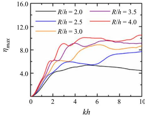
Figure 14. Frequency response of  $\eta_{max}$  for different values of  $R/h$ , with  $N = \infty$ ,  $r_0/R = 0.5$  and  $\text{Im}(\bar{c}) = 0$ .
