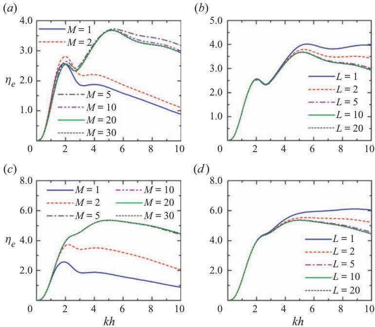
Figure 3. Frequency response of the wave power capture factor  $\eta_e$  for  $R/h = 2.0$ ,  $r_0/R = 0.5$ ,  $\beta = \pi/6$  and  $\bar{c} = 0.2$ : (a) impact of the angular cut-offs in terms of  $M$  for  $N = 4$  and  $L = 10$ ; (b) impact of the vertical cut-offs in terms of  $L$  for  $N = 4$  and  $M = 20$ ; (c) impact of the angular cut-offs in terms of  $M$  for  $N = \infty$  and  $L = 10$ ; (d) impact of the vertical cut-offs in terms of  $L$  for  $N = \infty$  and  $M = 20$ .
