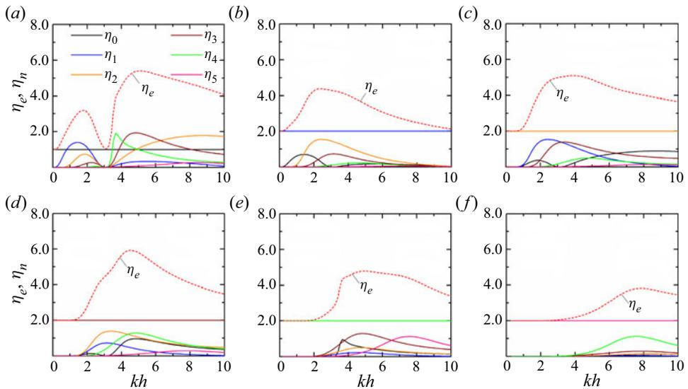
Figure 13. The partition of capture factor into contributions from different circular modes for operation tuned to be optimal for the  $m$ th mode, with  $R/h = 2.0$ ,  $r_0/R = 0.5$  and  $\beta = 0$ : (a)  $m = 0$ , (b)  $m = 1$ , (c)  $m = 2$ , (d)  $m = 3$ , (e)  $m = 4$ , and (f)  $m = 5$ .
