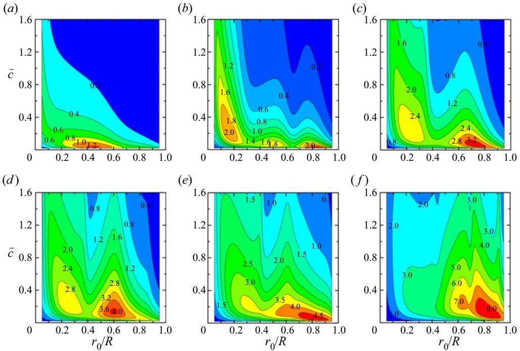
Figure 9. Contour plots for the variation of  $\eta_e$  as a function of PTO position  $r_0/R$  and PTO damping coefficient  $\bar{c}$ , for  $R/h = 2.0$ ,  $\beta = \pi/6$  and  $kh = 4.0$ : (a)  $N = 1$ ; (b)  $N = 2$ , (c)  $N = 3$ , (d)  $N = 4$ , (e)  $N = 5$ , and (f)  $N = \infty$ .
