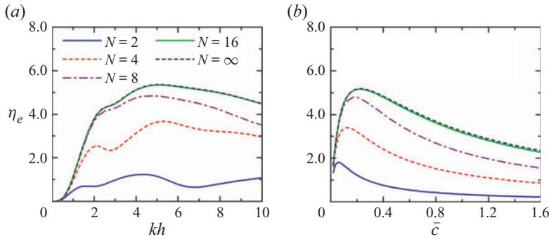
Figure 5. Comparison of the wave power capture factors of the devices with discrete and continuum PTO systems, with  $R/h = 2.0$ ,  $r_0/R = 0.5$  and  $\beta = \pi/6$ : (a) frequency response of  $\eta_e$  for  $\bar{c} = 0.2$ ; (b) variation of  $\eta_e$  with  $\bar{c}$  for  $kh = 4.0$ .
