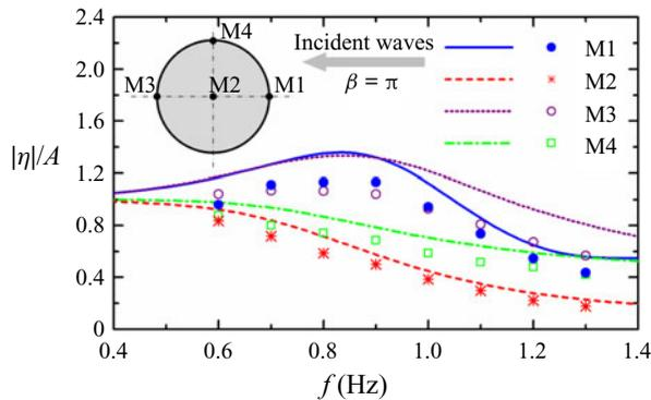
Figure 4. Deflection of four markers (M1–M4) placed on a free-floating elastic disk with  $R = 0.72$  m,  $h = 1.9$  m,  $\bar{\chi} = 3.55 \times 10^{-4}$  and  $\bar{\gamma} = 2.79 \times 10^{-3}$  as a function of frequency. Lines represent the present theoretical results with  $N = 4$ ,  $r_0/R = 0.5$ ,  $\bar{c} = 10^{-5}$ ; symbols represent the experimental data (Montiel *et al.* 2013b).
