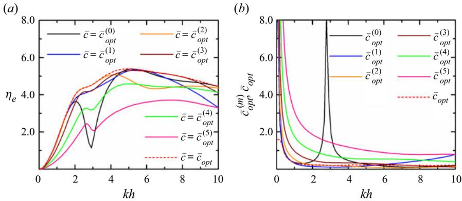
Figure 10. (a) Capture factor against dimensionless wavenumber for  $R/h = 2.0$ ,  $r_0/R = 0.5$ ,  $\beta = 0$  and  $\text{Im}(\bar{c}) = 0$ , with (b) corresponding damper values optimised in order to capture the available power in the  $m$ th circular mode component as much as possible.
