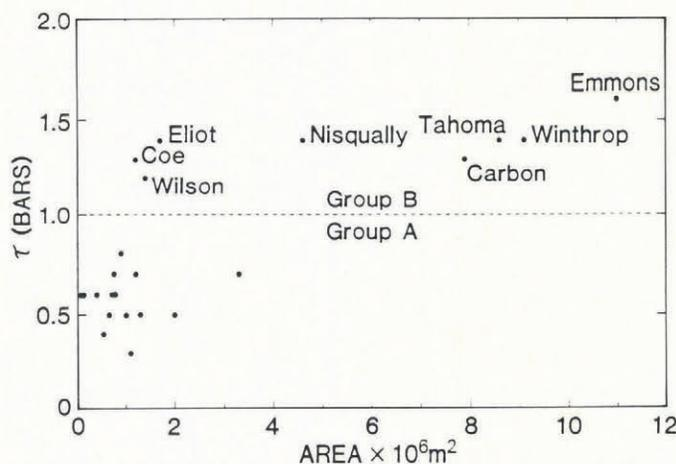
Fig.2. The graph illustrates a calculated basal shear stress versus area for glaciers in the Cascade volcano study.
