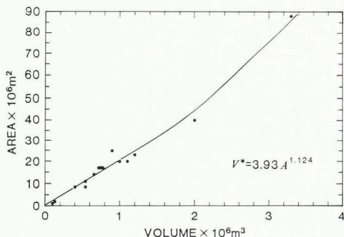
Fig.3. The graph illustrates the power curve  $V = 3.93A^{1.124}$ , derived when area is plotted against measured volume for smaller (group A) glaciers in the Cascades.
