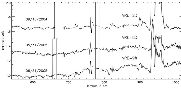
**Figure 3.** Surface reflectance SR( $\lambda$ ) (i.e. ER( $\lambda$ ) corrected from atmospheric absorption lines of  $O_2$ ,  $O_3$  and  $H_2O$ , and from Rayleigh scattering). Vertical lines define the spectral domains used for the VRE measurement. The plots have been shifted vertically for clarity.
