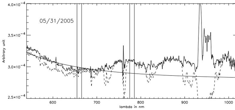
**Figure 2.** ER( $\lambda$ ) spectrum (dotted line) and SR( $\lambda$ ) obtained after removal of atmospheric (also called 'telluric') absorption lines but still showing the Rayleigh scattering. Smooth line is the fitted Rayleigh law. Vertical lines define the spectral domains used for the VRE measurement.
