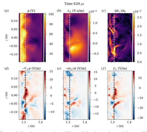
FIGURE 5. Snapshots (at z = 0,  $t = 620 \,\mu$ s) of the electrostatic potential  $\phi$ , parallel magnetic vector potential  $A_{\parallel}$  and normalized magnetic fluctuation amplitude  $|\delta B_{\perp}|/B_0 = |\nabla_{\perp}A_{\parallel}|/B_0 (a-c)$ , along with the components of the parallel electric field  $E_{\parallel} = -\nabla_{\parallel}\phi - \partial A_{\parallel}/\partial t (d-f)$ .
