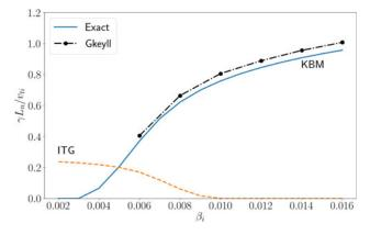
FIGURE 3. Growth rates for the KBM instability in the local limit, as a function of  $\beta_i$ , with  $k_{\perp}\rho_i = 0.5$ ,  $k_{\parallel}L_n = 0.1$ ,  $R/L_n = 5$ ,  $R/L_{Ti} = 12.5$ ,  $R/L_{Te} = 10$  and  $\tau = 1$ . The black dots are numerical results from Gkeyll, and the coloured lines are the result of numerically solving the analytic dispersion relation given by (5.6)–(5.7).
