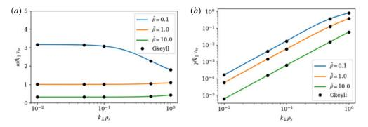
FIGURE 1. Real frequencies (a) and damping rates (b) for the kinetic Alfvén wave vs  $k_{\perp}\rho_s$ . Solid lines are the exact values from (5.5) for three different values of  $\hat{\beta} = (\beta_e/2)m_i/m_e$ , and black dots are the numerical results from Gkeyll.
