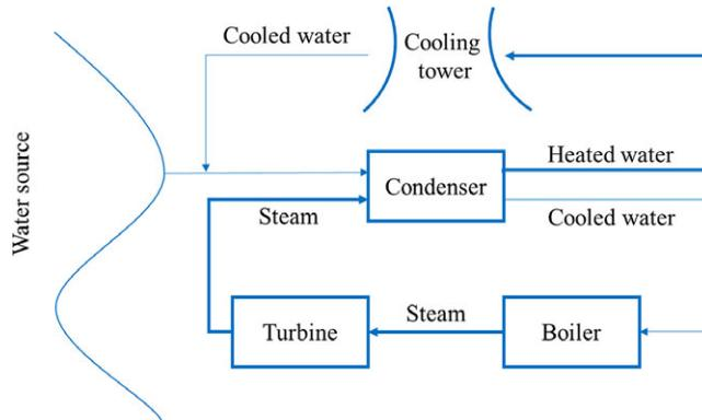
Figure 1. Recirculating cooling system with a cooling tower.
