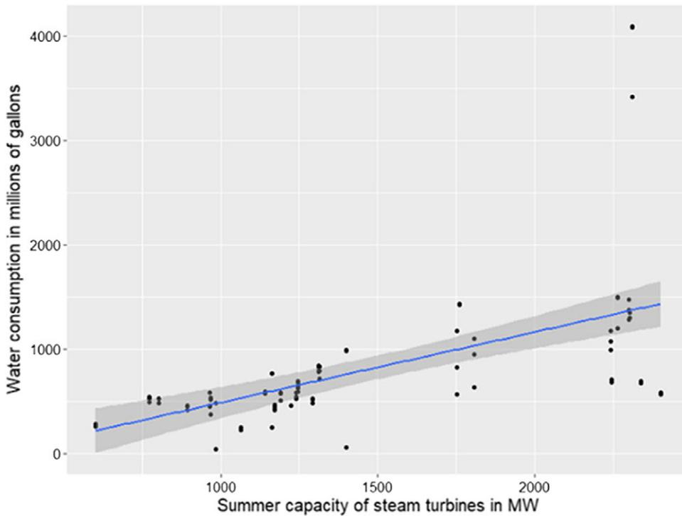
Figure 2. Water consumption in June, July, and August of 2019 across nuclear units with recirculating cooling systems. Each dot represents a particular month. Fitted line and 95% confidence interval from the simple OLS superimposed.
