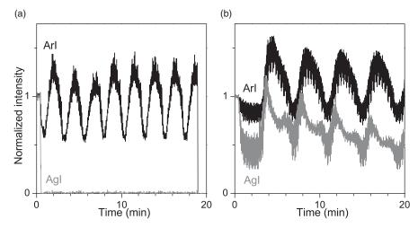
**Figure 1.** Time-resolved OES of argon (549.6 nm) and silver (546.5 nm) lines. Dust synthesis (a) without silver sputtering (P=10 W, HMDSO average flow = 0.28 sccm), and (b) with silver sputtering (P=30W, HMDSO average flow = 0.12 sccm).
