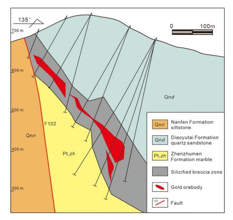
**Figure 4.** (Colour online) Cross-section showing the geology along exploration Line 34.
