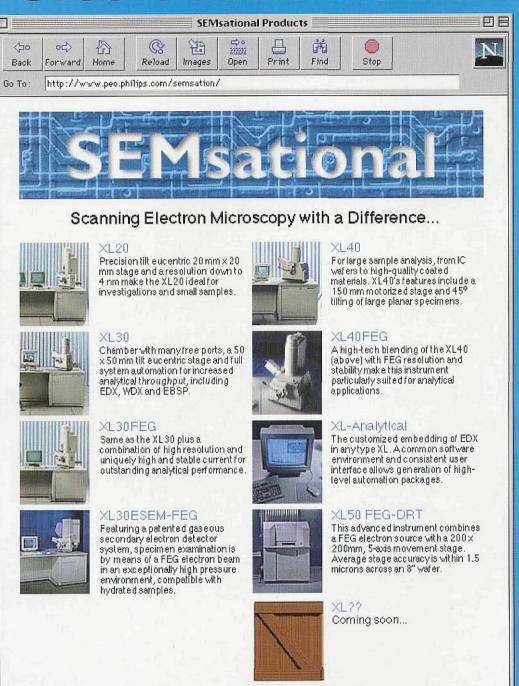
Philips XL Series SEMs reflect the perfect blend of elegant hardware and sophisticated software. System modularity and a choice of electron sources (tungsten; lanthanum hexaboride (LaB6), field emission (FEG)), enable a basic instrument to be configured to specific requirements. Menu-driven point-and-click mouse
