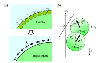
FIGURE 4. Fluid mechanical model of *Volvox*. (a) The colony is modelled as a rigid sphere, and forces generated by flagella are expressed by a shell of shear stress  $f_s$  at the distance  $\epsilon$  above the spherical surface. (b) Cartesian coordinate system used in the study, in which the gravity g acts in the  $e_3$  direction. A plane wall exists at  $e_3 = 0$ . The orientation vector of colony m is  $p^{(m)}$  that has the angle  $\theta_p^{(m)}$  from the  $e_3$  axis.
