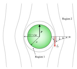
FIGURE 16. Schematic of the flow field around the 'shear-stress and no-slip' squirmer model. There is a no-slip spherical boundary at r=a, and uniform tangential stresses  $f_{\theta}$  and  $f_{\phi}$  are applied to the fluid at radius  $(1+\varepsilon)a$ . Region 1 is defined as  $a < r < (1+\varepsilon)a$ , whereas region 2 is defined as  $(1+\varepsilon)a < r$ .
