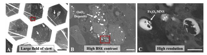
**Figure 2.** Backscattered electron images in SEM at 30kV highlighting a) the large field of view in SEM, where arrows indicate promising clusters of cells, b) high BSE contrast with clear osmium deposits and c) high resolution showing iron oxide MNS. Scale bars: a) 100  $\mu$ m, b) 5  $\mu$ m, c) 2  $\mu$ m.
