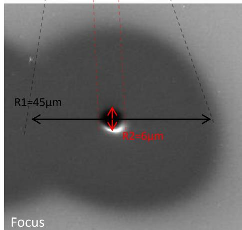
**Figure 1A Top:** AFM profile on top shows primary probe profile and extent of beam tail for under-focus condition. **Bottom:** SEM measurement of 1µA probe with 17.10KV objective voltage over focus setting. Primary probe radius measures 12µm with beam tail extending out to 26µm.
