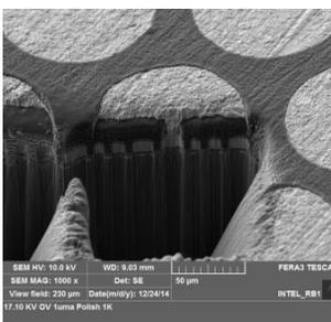
**Figure 2:** Shows comparison of locations milled using 1µA beam current at the focus setting of 17.25KV (2A left image) versus over-focus setting of 17.10KV (2B right image). Figure 2A shows the effect of extended beam tail with excessive material removal in the advance regions showing as compared with the more benign over focus setting.
