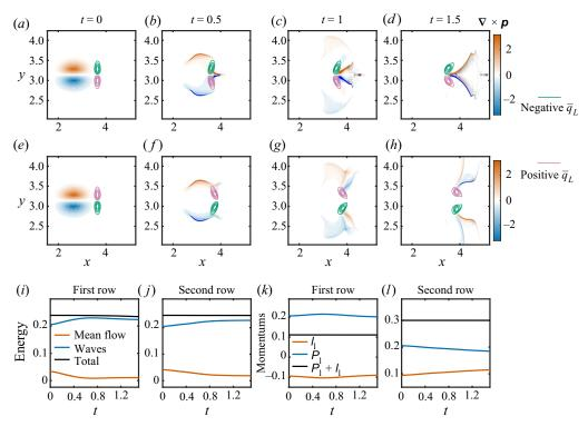
Figure 4. Simulations of wavepackets interacting with oncoming and retreating vortex couples (the sign of  $\bar{q}^L$  is flipped). In both,  $U_p = U_{\bar{q}^L} = 0.5$ . The plotted fields in (a-h) are  $\nabla \times p$  and  $\bar{q}^L$ , at t = 0, 0.5, 1, 1.5. Only a central region of the domain is shown. (i-l) The energies and momentum-like terms over time.
