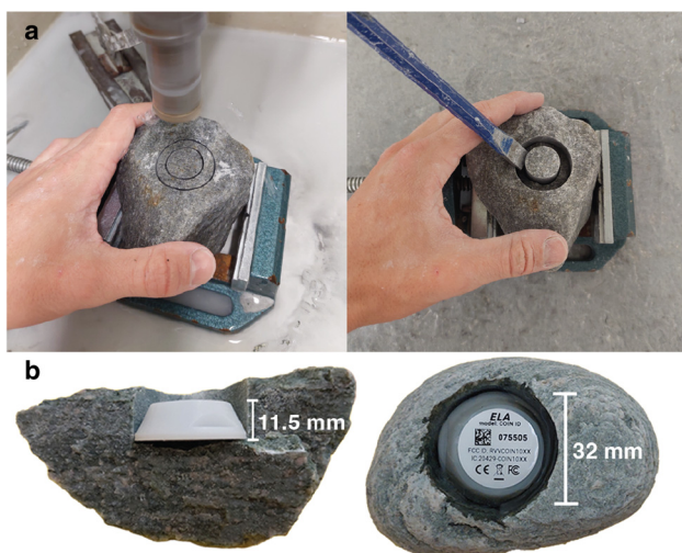
Figure 3. Tagging natural particles with active RFID transmitters. (a) Cavity creation with a drill press and diamond-tipped core bits. (b) Cross-section and top-down view of pebbles following transmitter insertion.
