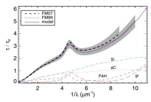
Figure 2. Mean extinction curve of the ISM by Fritzpatrick&Massa (2007, black) and a fit by the dust model of Sect. 2. Individual dust components are shown as labeled. The grey areas indicate the  $1\sigma$  deviation as of the samples.
