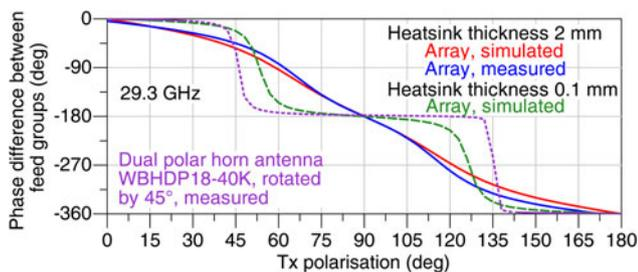
**Fig. 15.** Measured and simulated phase differences between the feed groups of the FE antenna and of a dual-polarized horn antenna for indicating nearly ideal behavior. The antenna-under-test was fixed and the illumination antenna is rotated around the boresight axis.
