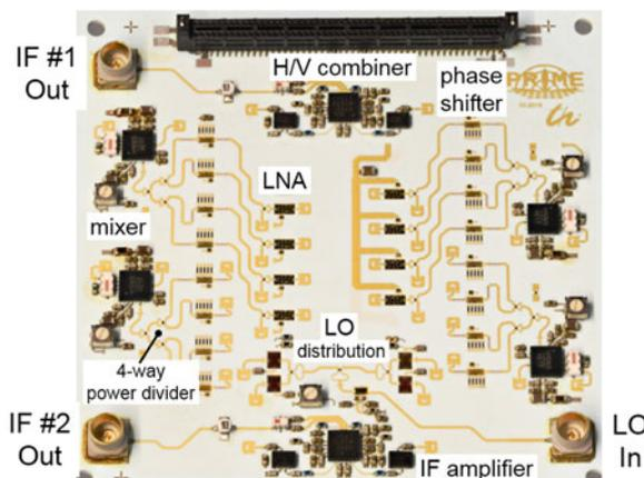
**Fig. 2.** Photograph of the assembled FE with SMP plugs for RF connections, and a power supply and control connector. The module size measures 74 mm × 74 mm [14].
