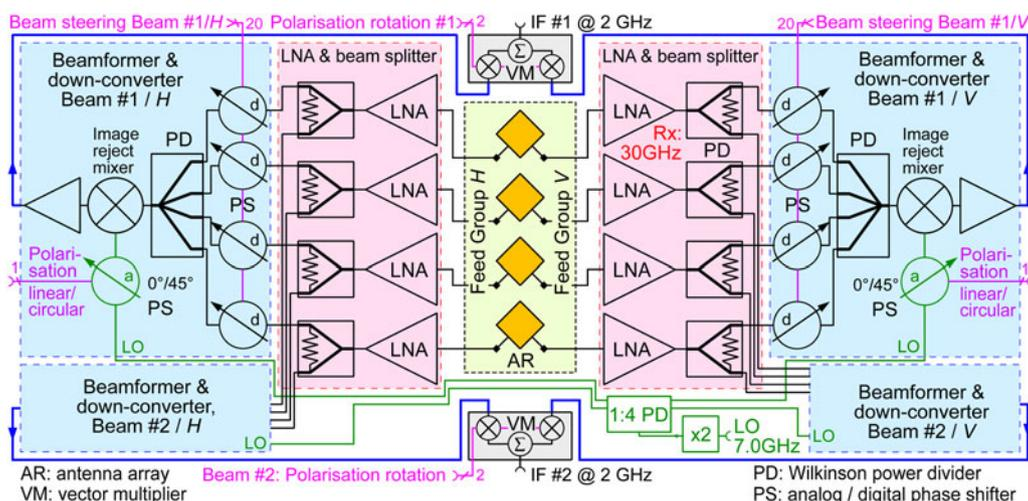
**Fig. 1.** Block diagram of the mm-wave FE with two steerable beams (beam #1 and beam #2 fed by the upper and lower parts of the circuit, respectively) and controllable polarization (H- and V-polarizations created in the left-hand and right-hand parts of the circuit, respectively). The beamformers and down-converters of beam #1 are shown explicitly, whereas the control circuits for beam #2 are indicated in a simplified way.
