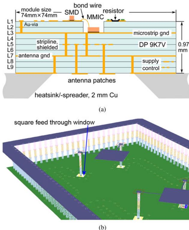
**Fig. 3.** Cross-section of the feedthroughs of the antenna signals of the multi-layer module mounted on a 2 mm copper heat sink, with microstrip and stripline structures on upper layers and the patch antenna array surrounded by the chamfered faces of the heat sink aperture (a) [12]. 3D view on the patch antennas with  $\lambda/4$ -transformers and vias for signal feed into the stripline plane (b).
