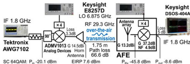
**Fig. 16.** OTA digital data transmission measurement setup.
