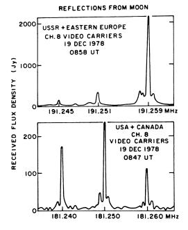
Figure 2. Video carriers of television transmitters observed after reflection off the moon. Resolution is 0.3 kHz.
