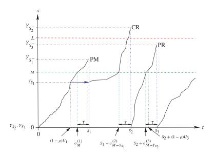
FIGURE 1: The condition-based maintenance policy.
