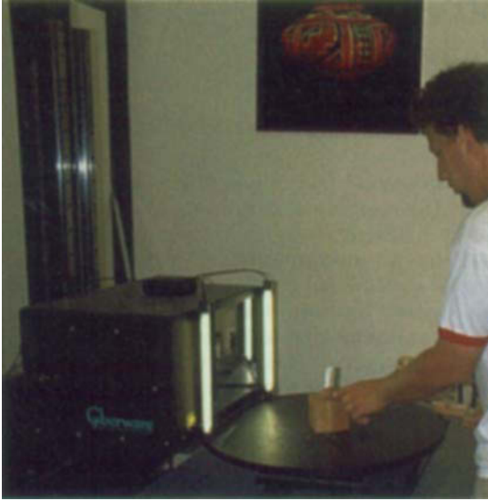
FIGURE 1 (left). 3D scanner with artefact; a researcher indicates where the laser hits the object.
