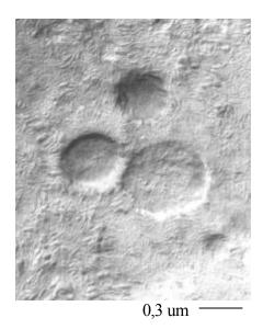
Figure 1. TEM permanganic etching followed by replication, LLDPE/iPP
