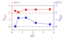
Figure 11. Integrated energy spectra of u'  $(I_{\phi_{u'u'}}, ----, \text{red})$  and  $\tilde{U}$   $(I_{\phi_{\tilde{U}\tilde{U}}}, ----, \text{blue})$  as a function of  $S/\bar{\delta}$  for SR cases. Red and blue dashed lines are  $I_{\phi_{u'u'}}$  and  $I_{\phi_{\tilde{U}\tilde{U}}}$  for the reference smooth wall SW-2, respectively.
