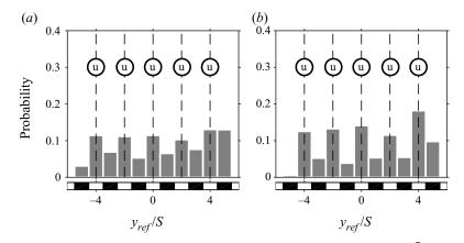
Figure 17. Histogram of the minima detected low-speed structures  $y_{ref}$  for case SR25 ( $z/\bar{\delta} = 0.18$ ): (a) large scales (figure 16a) and (b) small scales (figure 16b). Dashed lines (black dashed line) are the spanwise locations of the common flow up of the secondary flows (marked by  $(\mathbf{u})$ ).
