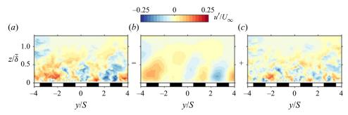
Figure 14. Turbulent velocity fluctuations u' of case SR25 in the *y*-*z*-plane: (*a*) all resolved scales, (*b*) large scales (constructed from u' POD modes with dominant  $\lambda_y/\bar{\delta} > 0.64$ ), (*c*) small scales (constructed from u' POD modes with dominant  $\lambda_y/\bar{\delta} \le 0.64$ ).
