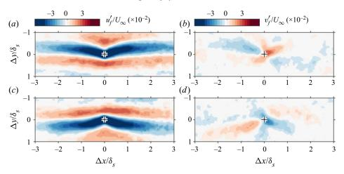
Figure 6. Contours of filtered turbulent fluctuation (a,c)  $u'_f$  and (b,d)  $v'_f$  conditionally averaged at (a,b) the minima and (c,d) maxima of the detected low-speed structures illustrated in figure 3 for the reference case SW-2 at  $z/\delta_s = 0.46$ . (a) SW-2. (b) SR250-2  $(S/\overline{\delta} = 3.63)$ . (c) SR160  $(S/\overline{\delta} = 2.28)$ . (d) SR100  $(S/\overline{\delta} = 1.35)$ . (e) SR50  $(S/\overline{\delta} = 0.62)$ . (f) SR25  $(S/\overline{\delta} = 0.32)$ .
