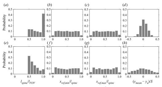
Figure 21. Histograms of the low-speed structures for case SR50 ( $S/\bar{\delta} = 0.62$ ), detected in the fluctuating velocity field:  $(a-d) \tilde{u}'$  and (e-h) u'. (a,e) Length of spines of the detected structures relative to the FOV, (b,f) streamwise position of the detected minima and (c,g) maxima relative to the length of the spines, (d,h) spanwise position of the spines relative to the common flow up.
