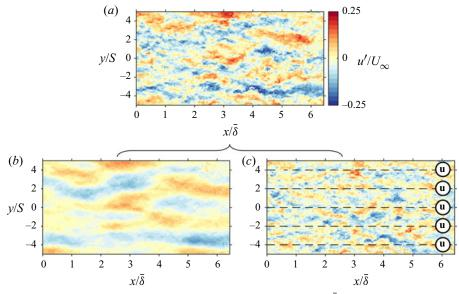
Figure 15. Turbulent velocity fluctuations u' of case SR25 in *x*-*y*-plane ( $z/\bar{\delta} = 0.18$ ): (*a*) all resolved scales, (*b*) large scales (constructed from u' POD modes with dominant  $\lambda_y/\bar{\delta} > 0.64$ ), (*c*) small scales (constructed from u' POD modes with dominant  $\lambda_y/\bar{\delta} \le 0.64$ ).
