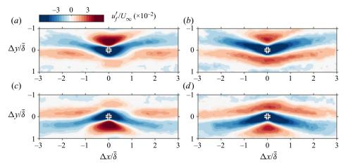
Figure 22. Contours of filtered turbulent fluctuation  $u'_f$  conditionally averaged at (a,b) the minima and (c,d) maxima of the detected low-speed structures for case SR50  $(S/\bar{\delta} = 0.62)$ . Structures are detected in the fluctuating velocity field:  $(a,c) \tilde{u}'$  and (b,d) u', as illustrated in figure 20.
