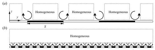
Figure 12. Illustration of the limiting cases in spanwise heterogeneous roughness: (a)  $S/\bar{\delta} \gg 1$  and (b)  $S/\bar{\delta} \ll 1$ . Areas bounded by black dotted line show regions approaching spanwise homogeneity.
