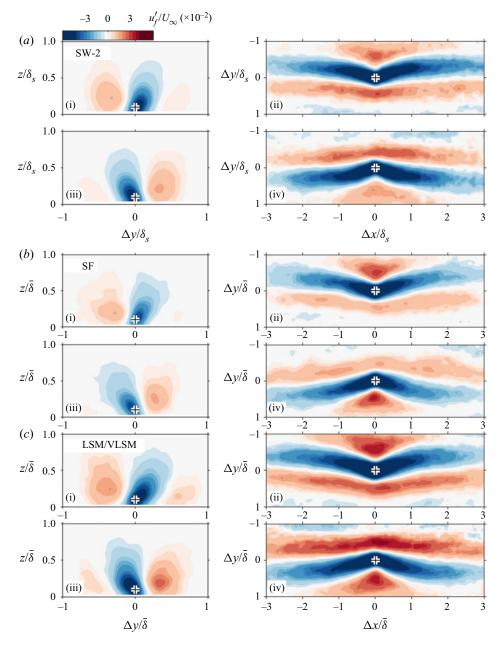
Figure 13. Contours of conditionally averaged turbulent fluctuation u' for (a) reference case SW-2 at  $z/\delta_s = 0.46$  and (b,c) SR250-2: conditioned at low-speed structures associated with (b) secondary flows (SF) and (c) LSMs/VLSMs. Conditions: (i)  $\tilde{u}' < 0$  and v' > 0, (iii)  $\tilde{u}' < 0$  and v' < 0, (ii) y-minima and (iv) y-maxima of detected spine-fitted low-speed structures ( $\tilde{u}'/U_{\infty} < -0.03$ ) illustrated in figure 3(b).
