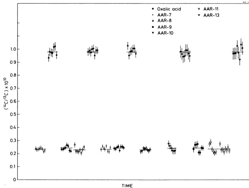
Fig 3.  $^{14}\text{C}/^{13}\text{C}$  ratios measured in 5 runs on the oxalic acid standard and 10 runs on different shell samples. The  $^{14}\text{C}/^{13}\text{C}$  ratio for the standard is constant within the statistical uncertainty and the isotopic ratio for the different shell samples are identical within the experimental errors.
