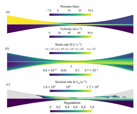
Figure 6. Simulation results for the flow of PEO 1000k solution at 140 ml h<sup>-1</sup> through the fused glass capillary geometry. Magnification from full computation mesh. Flow from left to right.
