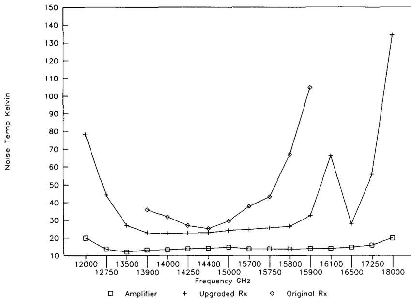
Fig. 2. Noise performance of cryogenic  $K_u$ -band amplifier and receiver. The noise performance of the same receiver with the narrow band amplifier is also shown.
