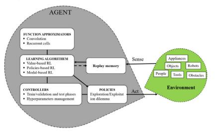
Fig. 10. General schematic of deep RL methods.<sup>172</sup>
