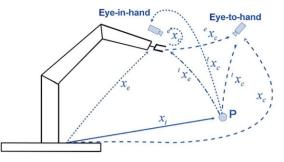
Fig. 4. Eye-in-hand and eye-to-hand configuration (adopted from ref. [49]).
