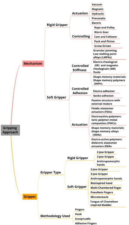
Fig. 11. Hierarchical structure of the grasping mechanism based on the gripping approach.
