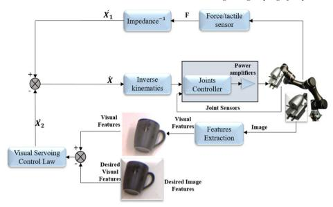
Fig. 6. Visual/force impedance control system (adopted from ref. [1]).
