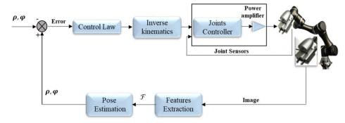
Fig. 3. Block diagram of visual servo system (adopted from ref. [1]).
