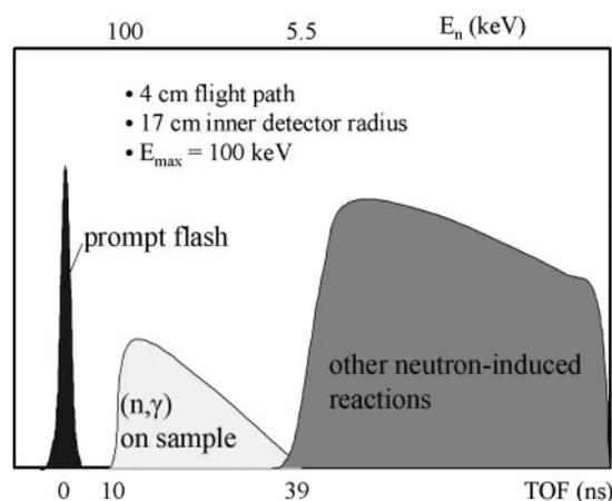
**Figure 6** Schematic TOF spectrum of the setup shown in Figure 3 similar to the one shown in Figure 4. In this case a very short flight path of only 4 cm was assumed. The intrinsic time resolution of the  $\text{BaF}_2$  array and the proton accelerator would be sufficient to disentangle neutron-capture events from neutron-induced background as well as from the  $\gamma$ -flash based on their time relative to the proton pulse.
