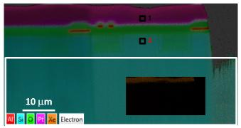
**Figure 1** shows an electron image and X-ray map of the lamella prepared in Xe plasma FIB. The inset shows the Xe map. The large rectangle indicates the area over which the thickness was mapped (figure 2). The small squares indicate area from which spectra were taken for the Xe implantation measurements (figure 3).
