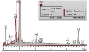
**Figure 3** shows two X-ray spectra (1) and (2). (1) is from the Pt rich top layer and (2) from an area just below containing only Si. The Cu and Al peaks are stray X-rays from the sample holder and grid post.
