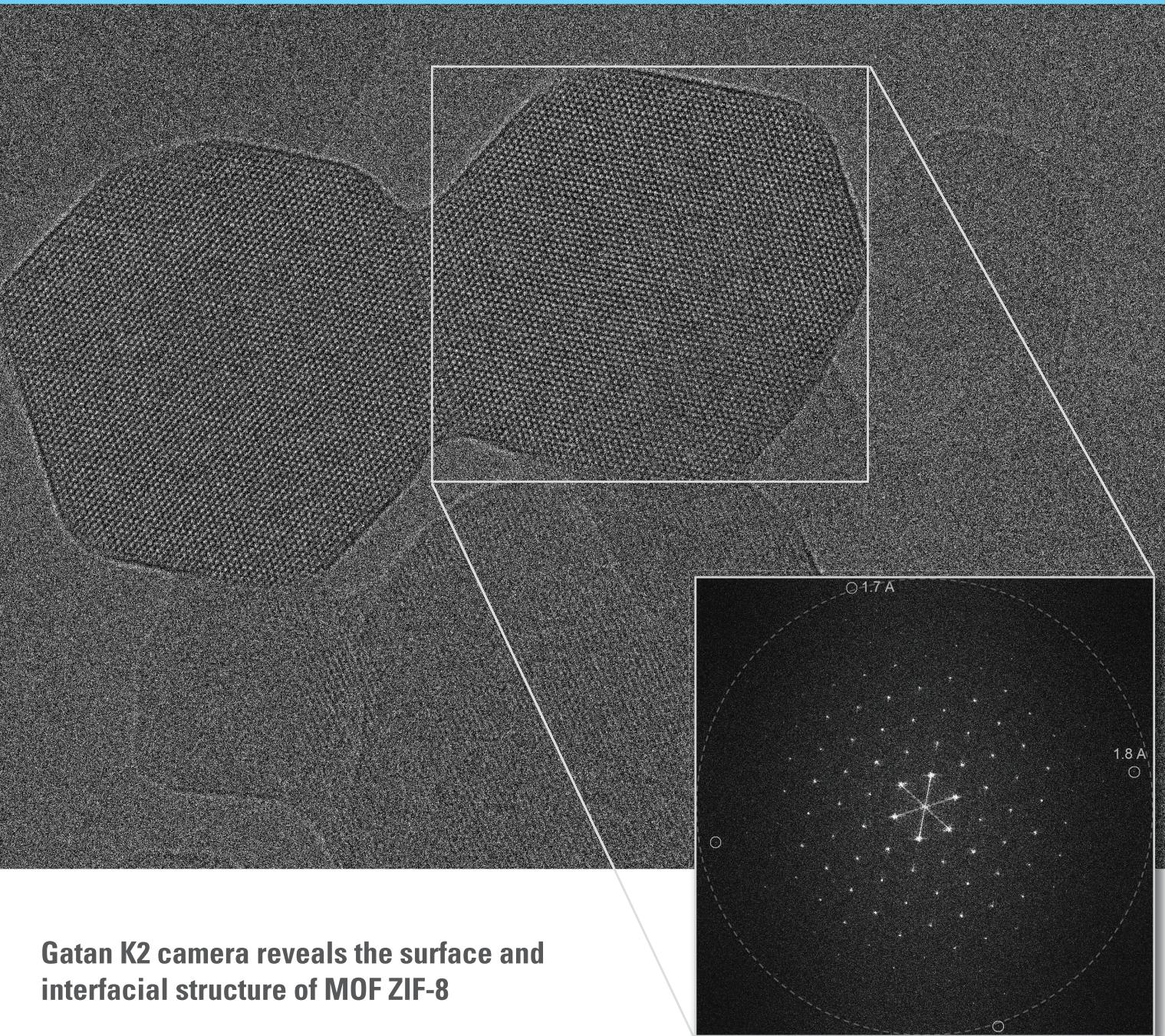
**Gatan K2 camera reveals the surface and interfacial structure of MOF ZIF-8**
