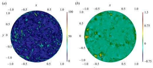
Figure 2. Visualization of the vorticity amplitude of  $\omega$  (*a*) and  $\mathscr{D}_{\ell}^{I}$  (*b*) for  $\ell = 8\eta$  on a plane containing the centre perpendicular to the cylinder's axis from the DNS of table 1.
