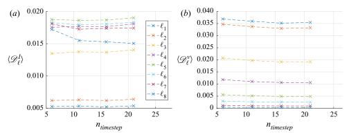
Figure 15. Convergence of mean DNS quantities for the 8 scales  $(\ell_1 < \ell_2 < \cdots < \ell_8)$  presented in figure 9(*a*) computed on 6, 11, 16 or 21 snapshots. (*a*)  $\langle \mathscr{D}_{\ell}^{\nu} \rangle$ .
