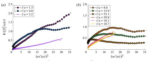
Figure 6. Conditional average  $\mathbb{E}(\mathscr{D}_{\ell}^{I}|\omega)/\epsilon$  as a function of  $(\omega/\langle\omega\rangle)^{2}$  for different scales  $\ell$ . They are computed from joint PDFs as in figures 3 and 4 from datasets of the DNS and cases T-1 to T-4 in table 1. Symbols are coded according to table 1.
