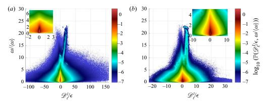
Figure 4. Joint PDF of  $\mathbb{P}(\mathscr{D}^{I}_{\ell}/\epsilon, \omega/\langle \omega \rangle)$  for different scales from the DNS in table 1 computed over 21 uncorrelated snapshots. Here,  $\omega$  refers to the norm of the vorticity, and  $\mathscr{D}^{I}_{\ell}$  is the energy transfer. A zoom on the central region is presented in each panel to compare with figure 3. (a)  $\ell = 1.06\eta$ ; (b)  $\ell = 26.5\eta$ . White colour corresponds to lack of events in the dataset.
