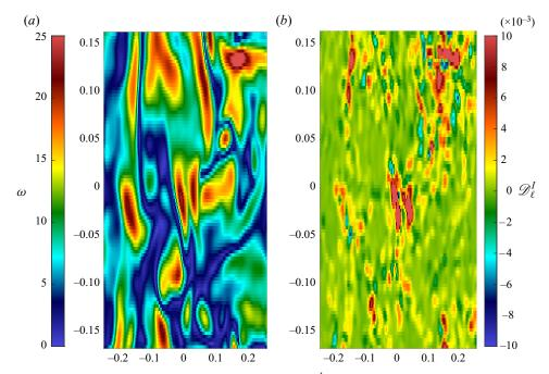
Figure 1. Visualization of the vorticity amplitude  $\omega$  (*a*) and  $\mathscr{D}_{\ell}^{I}$  (*b*) for  $\ell = 3.2\eta$  for the case T-4 of table 1 in a plane containing the cylinder's axis.
