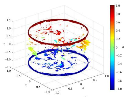
Figure 5. Positions of DNS points in the tail of figure 4(b) where  $\mathscr{D}_{\ell}^{I} > \epsilon$  and  $\omega > 5\langle \omega \rangle$  for  $\ell = 26.5\eta$ . The colours correspond to the z values of the points, indicating that most of them are close to the impellers (0.7 < |z| < 1.02), or at the tank mid-height. This plot shows positions for one single snapshot.
