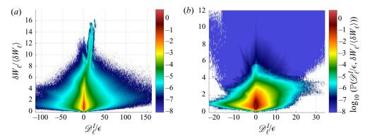
Figure 7. Joint PDF of  $\mathbb{P}(\mathcal{D}_{\ell}^{1}/\epsilon, \delta W_{\ell}/\langle \delta W_{\ell} \rangle)$  for different scales from the DNS in table 1 computed over 21 uncorrelated snapshots. (a)  $\ell = 1.06\eta$ ; (b)  $\ell = 26.5\eta$ . White colour corresponds to lack of events in the dataset.
