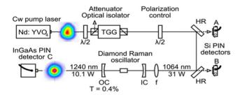
**Figure 4.** Schema of the external cavity DRL<sup>[3]</sup>.
