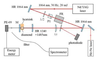
**Figure 3.** Schematic of the external cavity Raman laser<sup>[67]</sup>.
