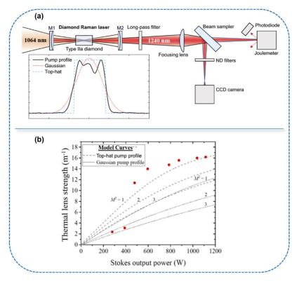
**Figure 10.** High-power DRL pumped by Nd:YAG pulsed laser<sup>[107]</sup>: (a) experimental setup of the DRL and output beam characteristics; (b) thermal lens strength as a function of Stokes output power.
