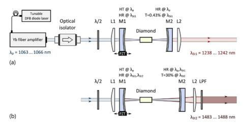
Figure 6. Experimental setup of the tunable (a) first-order and (b) second-order Stokes DRL operating in SLM<sup>[70]</sup>.
