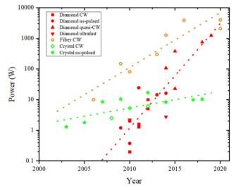
**Figure 1.** Achieved output power of DRLs<sup>[8,23,28–43]</sup> compared with other crystalline Raman lasers<sup>[33,44–53]</sup> and Raman fiber lasers<sup>[54–61]</sup>.
