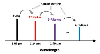
**Figure 8.** Schematic of a cascaded DRL pumped by a 1.06  $\mu$ m laser<sup>[20]</sup>.
