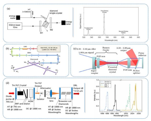
**Figure 9.** Different wave bands of DRLs and the related output spectra<sup>[7,90–92]</sup>: (a) 573 nm and 620 nm laser output from 532 nm pump beam; (b) 275.7 nm laser output from 266 nm pump beam; (c) 3.38–3.8  $\mu$ m laser output from 2.33–2.52  $\mu$ m pump beam; (d) ~2.53  $\mu$ m laser output from 1.89  $\mu$ m pump beam.
