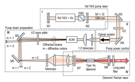
Figure 5. Layout of the external cavity DRL pumped with a Nd:YAG pulsed laser<sup>[40]</sup>.
