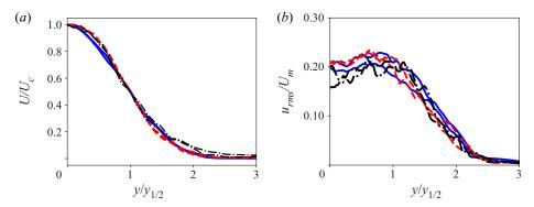
Figure 14. Spanwise profiles of (a) mean streamwise velocity  $(U/U_c)$  and (b) fluctuations  $(u_{rms}/U_c)$ . Here, S/d = 2, x/d = 30, 40 (——, blue); S/d = 4, x/d = 45, 50 (——, red); S/d = 8, x/d = 70, 80 (——).
