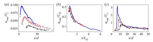
Figure 13. Development of streamwise velocity fluctuations along configuration axis y = 0, z = 0 from LES (a) scaled with  $U_i$  and  $U_i$ , (b) scaled with  $U_i$  and  $U_i$ , (c) scaled with  $U_i$ . Here,  $U_i$ , blue),  $U_i$ ,  $U_i$ , red),  $U_i$ ,  $U_i$ ,
