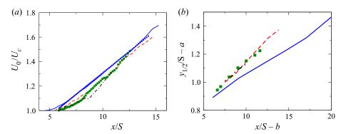
Figure 15. Development of (a) mean centreline velocity and (b) half-width. Here, S/d=2 (——, blue), 4(---, red),  $5(\blacksquare, \text{green})$ ,  $8(-\bullet-\bullet)$ . Linear fit to the velocity development for S/d=2 in panel (a) above is shown as a dotted line. Curves in panel (b) have been translated to show the nearly similar development for S/d=4, 5, 8.
