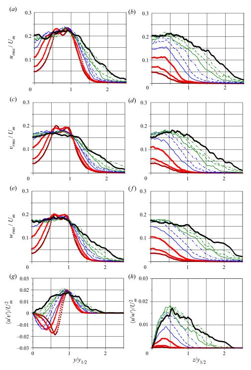
Figure 9. (a-f) Fluctuation profiles and (g,h) Reynolds shear stress profiles. All are normalized with maximum of local mean streamwise velocity  $U_m$  and distance  $y_{1/2}$ . Here, x/d=8 ( $\circ$ , red), 10 ( $\bullet$ , red), 15 ( $\blacksquare$ , red), 20 ( $\longrightarrow$ , blue), 25 (--, blue), 30 ( $-\bullet$ , blue), 35 ( $\longrightarrow$ , green), 40 (--, green), 45 ( $-\bullet$ , green), 50 ( $-\circ$ ).
