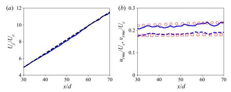
Figure 1. Self-preservation in mean and fluctuations of velocity in a single round jet at  $Re = 11\,000$  compared with the experiment of Panchapakesan & Lumley (1993). (a) Reciprocal of centreline velocity: LES (——, blue); experiment (– – –, black). (b) Velocity fluctuations: LES,  $u_{rms}$  (——, blue); LES,  $v_{rms}$  (– – –, blue); experiment,  $u_{rms}$  ( $\circ$ , red); experiment,  $v_{rms}$  ( $\square$ , red).
