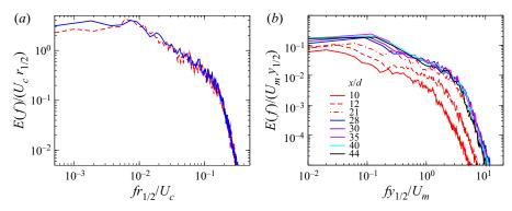
Figure 3. Power spectral density E(f) of streamwise velocity component u(x, 0, 0, t). Scaled with local scales  $U_c$  and  $r_{1/2}$  (case SR120), and  $U_m$  and  $y_{1/2}$  (case TR255). (a) Single jet, x/d = 35 (---, red), 48 (---, blue). (b) Twin jet.
