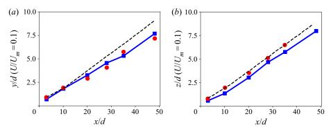
Figure 7. Jet spreading in two planes. Jet boundary is located where mean velocity U is 10 % of the maximum over cross-section (x, constant): experiment  $(\bullet, \text{red})$ ; LES  $(-\blacksquare -, \text{blue})$ ; single jet (---). (a) On z=0 and (b) on y=S/2.
