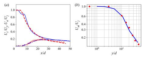
Figure 6. Development of mean streamwise velocity for case TR255. (a) Decay compared with measurement along nozzle axis:  $U_n$ , LES (——, blue);  $U_n$ , experiment (– –, red);  $U_c$ , LES (– • –, blue);  $U_c$ , experiment ( $\circ$ , red). (b) Maximum at any cross-section, initially within individual jets and along x-axis after jets merge:  $U_n$ , LES (——, blue);  $U_c$ , experiment ( $\bullet$ , red).
