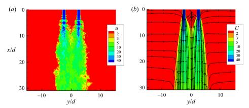
Figure 5. Streamwise component of velocity on plane z = 0 from LES of case TR255. (a) Streamwise velocity u(x, y, 0, t) (m s<sup>-1</sup>). (b) Mean streamwise velocity U(x, y, 0) (m s<sup>-1</sup>) and streamlines.
