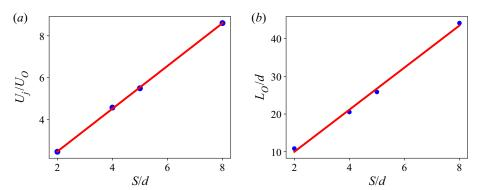
Figure 12. Dependence of intrinsic scales on nozzle spacing. (a) Maximum of centreline velocity,  $U_0$ . (b) Distance  $L_0$  from inflow plane. Here, LES ( $\bullet$ , blue); linear fit (——, red).
