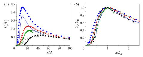
Figure 11. Development of streamwise velocity along configuration axis y=0, z=0 for  $2 \le S/d \le 8$ . (a) Scaled with input parameters;  $U_c(x)$ . (b) Scaled with peak velocity  $U_0$  and distance to peak  $U_0$ ;  $U_c(x)$  scaled with  $U_0$  and  $U_0$ . For LES:  $U_0$  for LES:  $U_0$  for  $U_0$ , blue),  $U_0$ ,  $U_0$ ,
