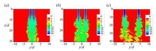
Figure 10. Streamwise component of velocity at an instant on plane z = 0 from LES at  $Re = 25\,000$ . (a) S/d = 2, (b) S/d = 4, (c) S/d = 8.
