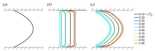
Figure 2. Schematic representation of the components of pulsating Poiseuille flow for  $\tilde{Q} = 0.6$  and Wo = 25 over one period (T = 75.4). The complete profile (c) is plane Poiseuille flow (a) superimposed with an oscillating flat Stokes layer (b).
