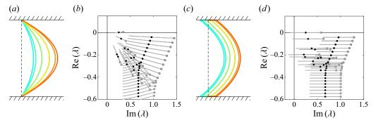
Figure 6. Base flow profiles and corresponding eigenorbits for extreme values of the Womersley number at  $\tilde{Q} = 0.5$ . In this parameter range there are no subharmonic eigenvalue orbits. Here (a,b) Wo = 0.1; (c,d) Wo = 300.
