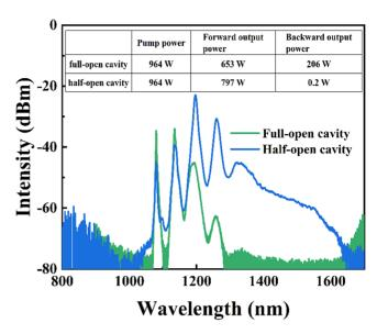
**Figure 4.** Compared output spectra of RFLs with a full-open cavity and a half-open cavity under the same pump power of 964 W.
