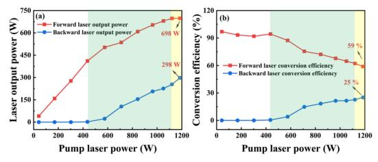
Figure 3. (a) Laser output power and (b) conversion efficiency of the RFL with a full-open cavity in both directions. The green background area is the growth area of the backward output power; the yellow background area shows that the forward output power stops increasing.
