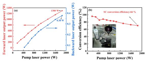
Figure 6. (a) Laser output power and (b) conversion efficiency in the RFL with a half-open cavity.
