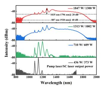
**Figure 5.** Output spectral evolution with pump laser power in the RFL with a half-open cavity.
