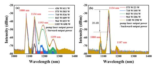
Figure 2. Output spectral evolution of pump laser power in the RFL with a full-open cavity: (a) forward direction and (b) backward direction.
