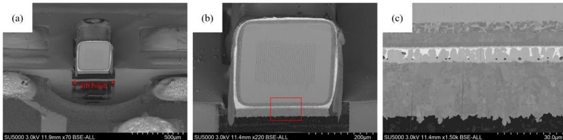
**Figure 2.** Results after FIB polishing; (a) Annotated cross section view a resistor collected at 3kV accelerating voltage and 70X magnification. (b) Annotated cross section view a resistor collected at 3kV accelerating voltage and 220X magnification. (c) Higher magnification investigation of the indicated portion of a resistor shown in (b) collected at 3kV accelerating voltage and 1,500X magnification.
