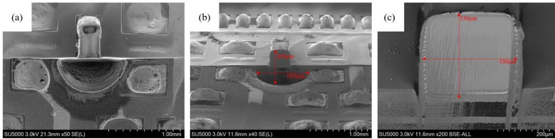
**Figure 1.** Results after BIB milling; (a) Top-down SEM image of a resistor cross section collected at 3kV accelerating voltage and 50X magnification. (b) Annotated cross section view of a resistor collected at 3kV accelerating voltage and 40X magnification. (c) Annotated cross section view of a resistor collected at 3kV accelerating voltage and 200X magnification.
