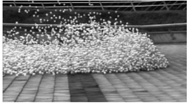
Fig. 5. Side view of the head of a 550 000 ball avalanche at the Miyanomori ski jump.
