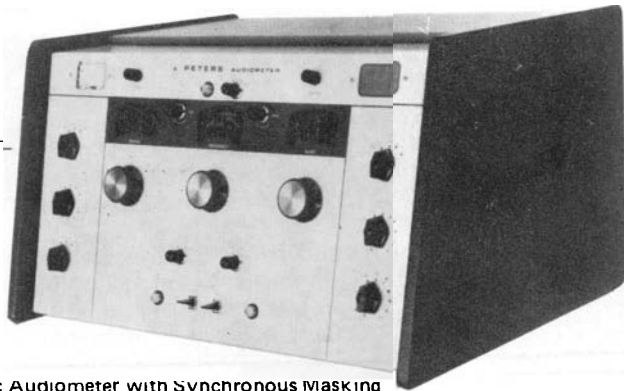
A Peters AP6 Clinic Audiometer with Synchronous Masking
