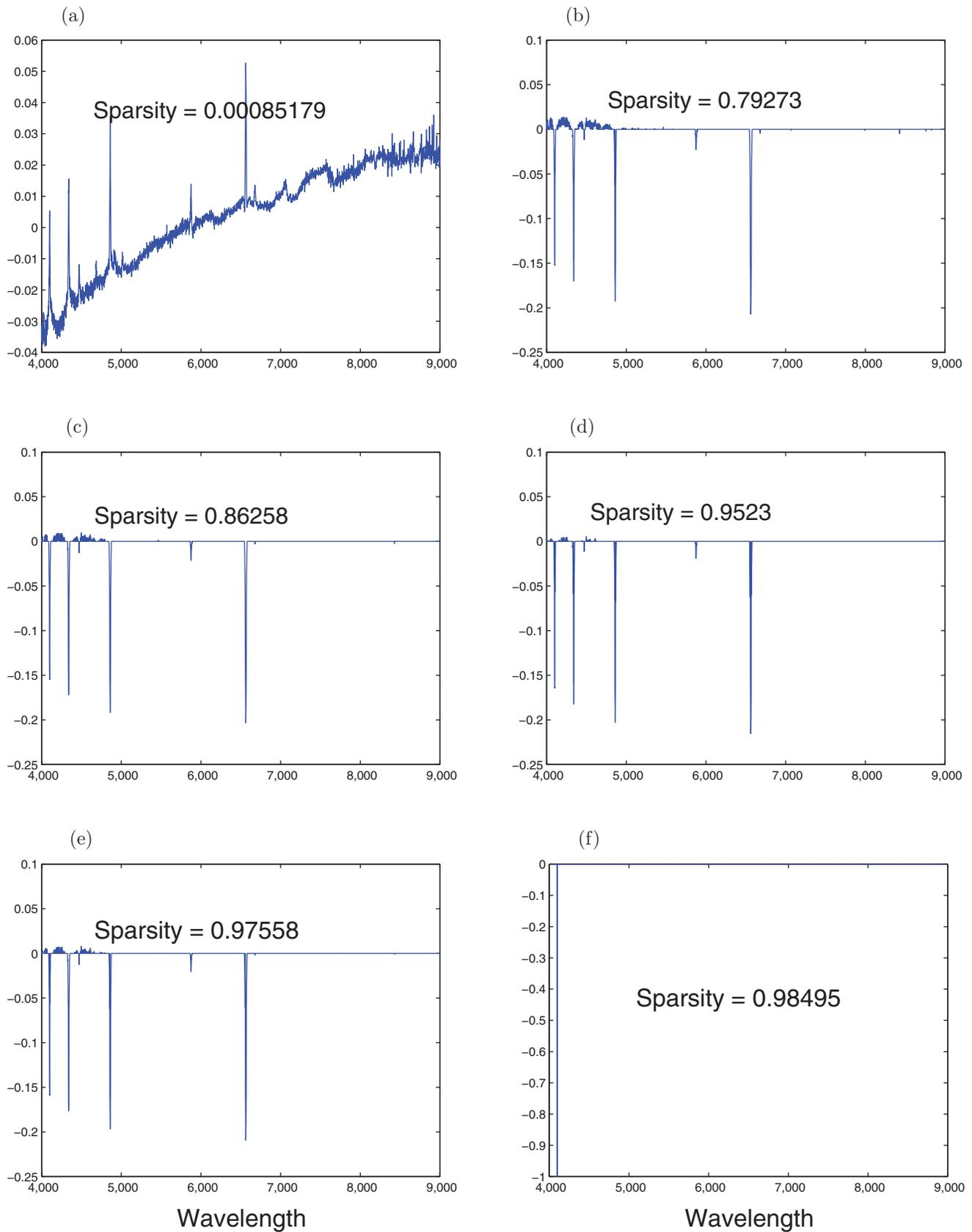
**Figure 7.** The first sparse eigenspectra with various sparsity. The spectral features will disappear if sparsity is above 0.98, while the redundant elements of the spectrum have not been reduced to zero if sparsity is below 0.95.
