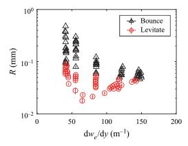
Figure 3. Phase diagram of the 100 cSt drops with a drop radius *R* versus concentration gradient  $dw_e/dy$  parameter space. Black triangles stand for bouncing drops, red circles for levitating ones. When experimentally determining the phase diagram, whether the drop bounces or not is decided within half an hour after its release to avoid any untraceable change of the gradient arising from long-term mixing induced by the drop motion itself.
