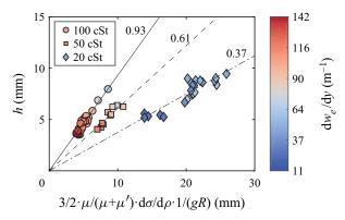
Figure 9. Levitation heights *h* of 100, 50 and 20 cSt silicone oil drops in linearly stratified ethanol–water mixtures with different concentration gradients  $dw_e/dy$ . The prefactors  $\alpha$  (defined in (A3)) are measured to be 0.93, 0.61 and 0.37 for 100, 50 and 20 cSt silicone oil drops, respectively.
