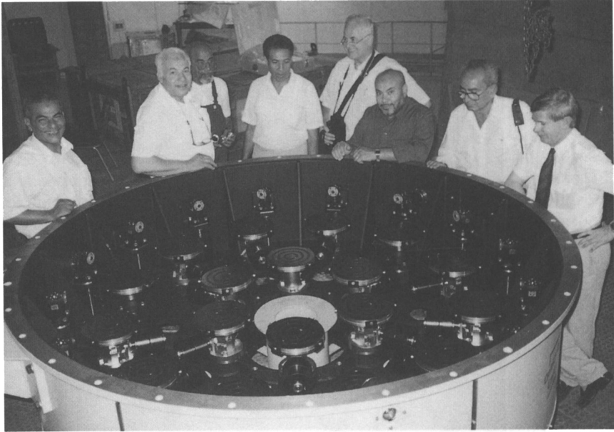
Figure 2. Distribution of the 18 axial supports in the modified cell
