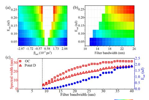
**Figure 6.** (a) FWHM spectral width of output pulses as a function of NCD and  $E_{\rm sat}$ . Linear scale: 4 nm 20 nm (white area: multi-pulsing region). (b) FWHM spectral width of pulses at point D as a function of filter bandwidth and  $E_{\rm sat}$ . Linear scale: 8 nm 16 nm (white area: multi-pulsing region). (c) FWHM spectral width of pulses at the OC (red open squares) and at point D (red open-triangles) at critical pump power and corresponding  $E_{\rm sat}$  (blue solid circles).
