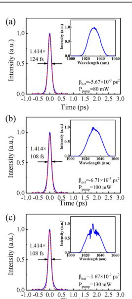
**Figure 4.** Autocorrelation traces of dechirped output pulses (blue solid lines) and Gaussian fitting curves (red dashed lines) at a pump power of (a) 80 mW, (b) 100 mW, and (c) 130 mW. Insets: corresponding spectra of output pulses.
