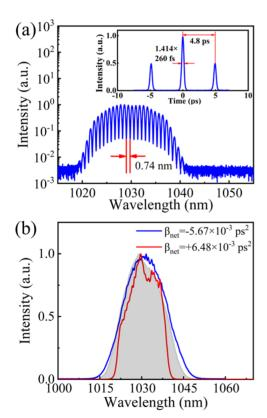
**Figure 3.** (a) Spectrum and autocorrelation trace of soliton molecules at 80 mW pump power. (b) Spectra of single soliton states for two critical NCD values at 80 mW pump power (gray area: CFBG reflection spectrum).
