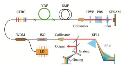
**Figure 1.** Experimental setup of the passively mode-locked all-PM fiber laser. LD, laser diode; WDM, wavelength division multiplexer; CFBG, chirped fiber Bragg grating; YDF, Yb-doped fiber; SMF, single-mode fiber; SESAM, semiconductor saturable absorber mirror; HWP, half-wave plate; PBS, polarization beam splitter; ISO, isolator.
