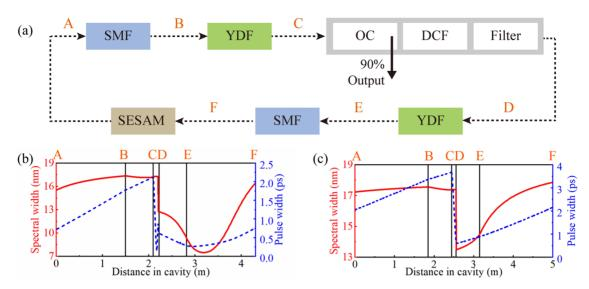
Figure 5. (a) Schematic of the numerical simulation model. Evolution of spectral width (red solid line) and temporal width (blue dotted line) when the NCD is for (b)  $\beta_{\text{net}} = -1.1 \times 10^{-3} \text{ ps}^2$  and (c)  $\beta_{\text{net}} = +1.5 \times 10^{-2} \text{ ps}^2$ . YDF, Yb-doped fiber; SMF, single-mode fiber; SESAM, semiconductor saturable absorber mirror; DCF, dispersion compensating fiber; OC, optical coupler.
