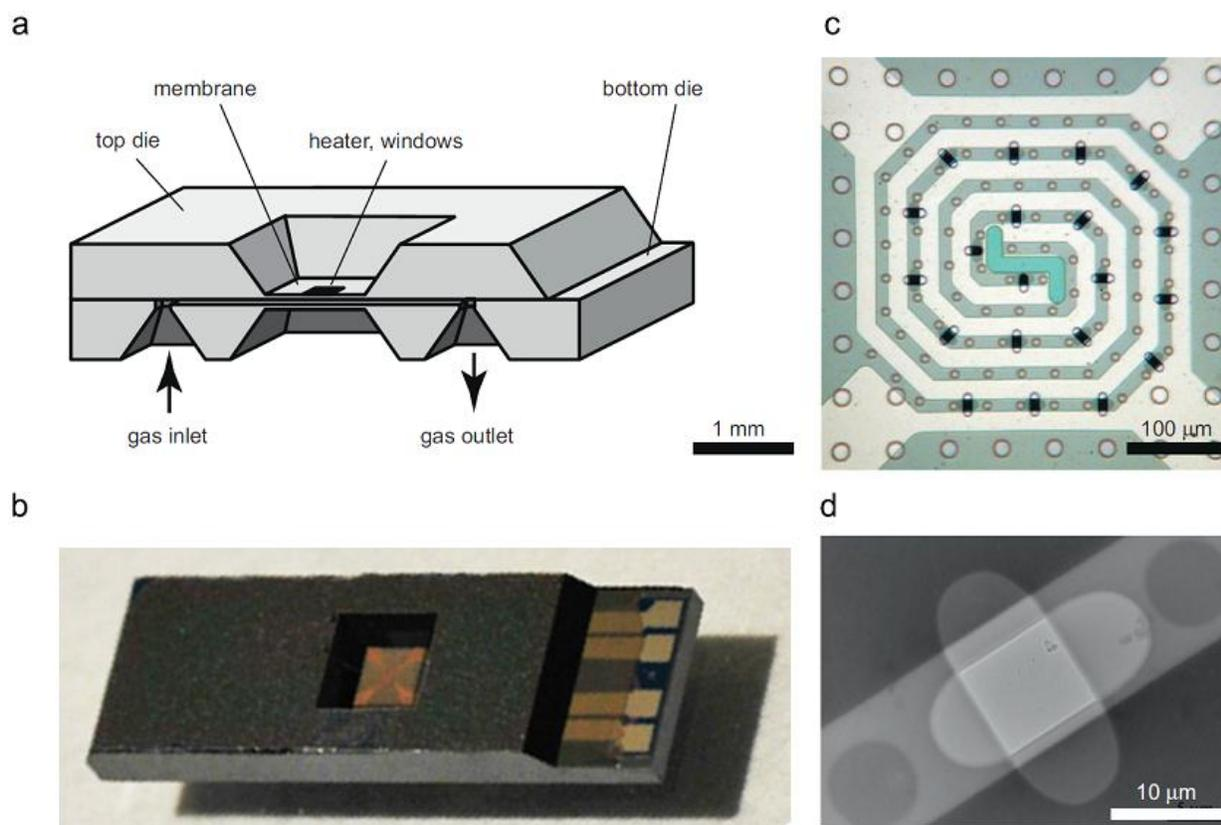
**Figure 1.** (a) Schematic cross-section of the nanoreactor. (b) Optical image of the nanoreactor. (c) Optical close-up of the nanoreactor membrane. The bright spiral is the heater. The small ovaloids are the electron-transparent windows. (d) A low-magnification TEM image of a pair of superimposed 10 nm thick windows creating highly electron-transparent areas for HRTEM.
