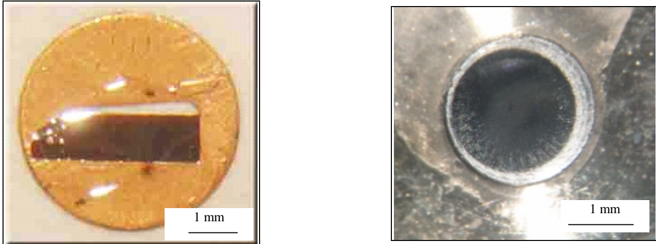
FIG.1. Optical micrograph showing a tripod polished sample (left) and a dimpled sample (right) following mechanical preparation. Both cross sectional and plan view samples can be prepared with these methods.
