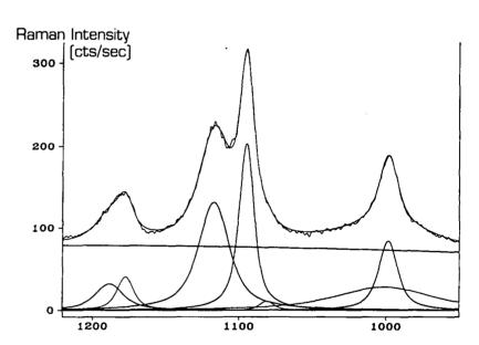
Raman shift (cm-1) Band Fit of Raman spectrum of glycol group in Polyethylene Terephthalate. Circle No. 15 on Reader Service Card.
