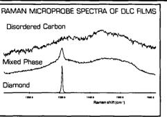
The Raman Microprobe MOLE° can tell ou what phase(s) of carbon is present n a matter of seconds:
