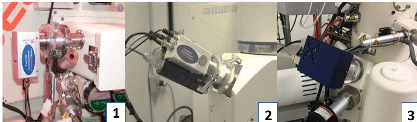
Figure 1. Three generations of Evactrons mounted on SEMs. 1) Evactron 10 PRS in 2004 first servo control of pressure, 2) Evactron 25 PRS with shroud over the valve manifold. 3) Evactron 50 PRS in 2018 high performance cleaning at 50 watts, external hollow cathode and lower cost.
