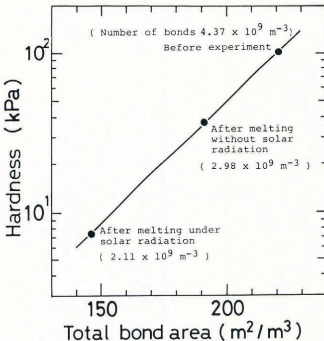
Fig. 4. Hardness and total bond area of the observation layer shown in Figure 3.
