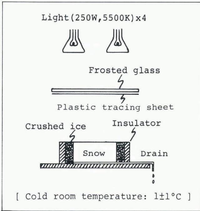
Fig. 2. Apparatus for laboratory experiments.
