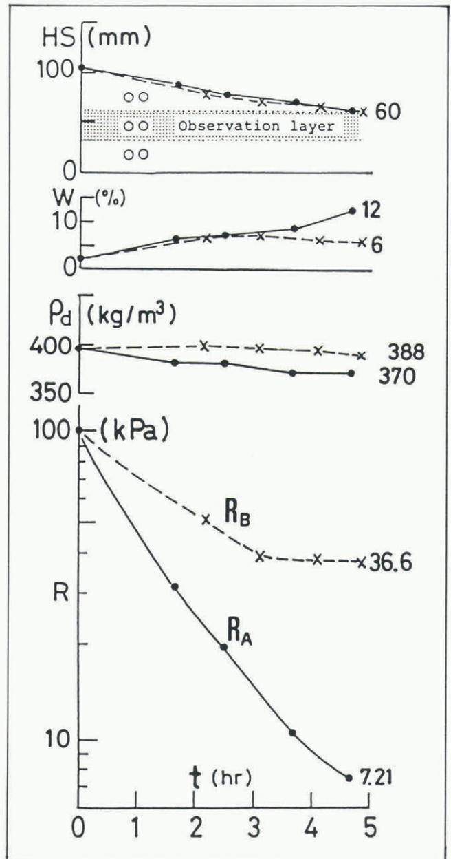
Fig. 3. Decrease in hardness,  $R$ , of snow at  $0^{\circ} \text{C}$ . Solid line: under solar radiation; dashed line: without solar radiation. HS: surface level of snow specimen;  $W$ : water content;  $\rho_d$ : dry density of snow.
