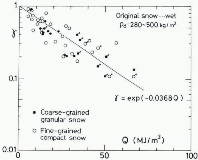
Fig. 5. Relationship between absorbed solar radiation,  $Q$ , and hardness ratio,  $\gamma$ . Circles with arrow: field experiments; circles without arrow: laboratory experiments.
