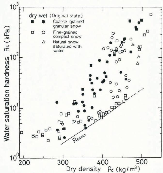
Fig. 1. Relationship between water saturation hardness,  $R_s$ , and original dry density,  $\rho_d$ .  $R_{s-min}$  indicates the lower limit of  $R_s$  values.
