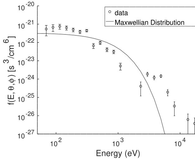
FIGURE 2. Measured ion velocity distribution function (circles) as a function of energy measured at fixed angles and at a given time, compared with the associated Maxwellian distribution (solid line). Error bars are also shown.
