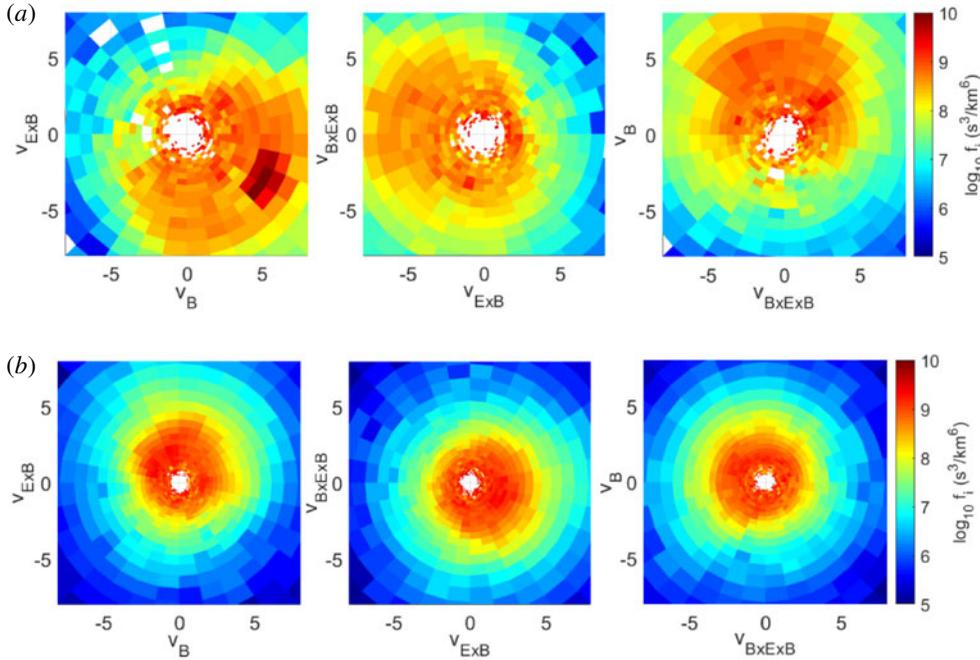
FIGURE 4. Two-dimensional VDF cuts in the two regions highlighted with vertical red dashed lines in figure 3. The top panels refer to a peak in  $\epsilon_i$ , while the bottom panels refer to a valley in  $\epsilon_i$ . Notice the presence of a particle beam almost aligned with the  $\mathbf{B}$  direction in the top panels. Velocity values are normalized to the local Alfvén speed.
