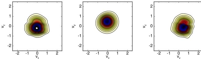
FIGURE 7. Two-dimensional VDF cuts in the portion of the signal highlighted in figure 6 by the vertical dashed line. A beam almost aligned with the  $\mathbf{B}_0$  direction is clearly visible.
